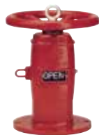
Series 34/80 Wall post indicator, for DN50-400 post indicator gate valves Stem length 250-1250 mm Ductile iron UL/ULC listed, FM approved
