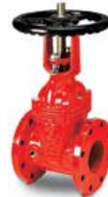
Series 45/56 Flanged gate valve with rising stem DN50-300: 17,2 bar (250 PSI) DN350-400: 13,7 bar (200 PSI) Ductile iron UL/ULC listed, FM approved
