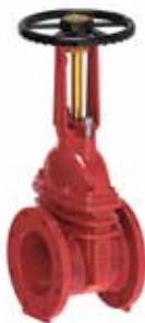
Series 145/46 Flanged gate valve with rising stem DN50-200 17,2 bar (250 PSI) Ductile iron UL/ULC listed, FM approved
