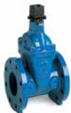
Series 45/59 Flanged gate valve with wrench nut DN50, 250 and 300: 17,2 bar (250 PSI) DN350-400: 13,7 bar (200 PSI) Ductile iron UL/ULC listed, FM approved
