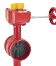
Series 815/40 Butterfly valve Centric with rubber Vulcanised disc Grooved ends to AWWA C606 DN65-200 24,1 bar (300 PSI) Ductile iron UL/ULC listed, FM approved
