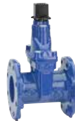
Series 145/50 Flanged gate valve with wrench nut DN65-200 17,2 bar (250 PSI) Ductile iron UL/ULC listed, FM approved
